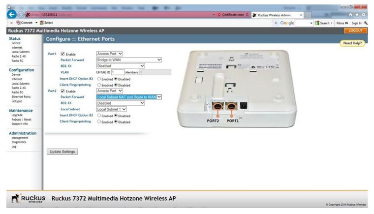
Disconnect the POE LAN cable from the Ruckus ZF 7372 to power it off. Reconnect the cable to the Ruckus ZF 7372. Go back to the Step 1.8 to reconnect to the Ruckus ZF 7372. After entering, check the changes made including in the Ethernet Ports, and press the LOGOUT button on the right upper corner to exit.
