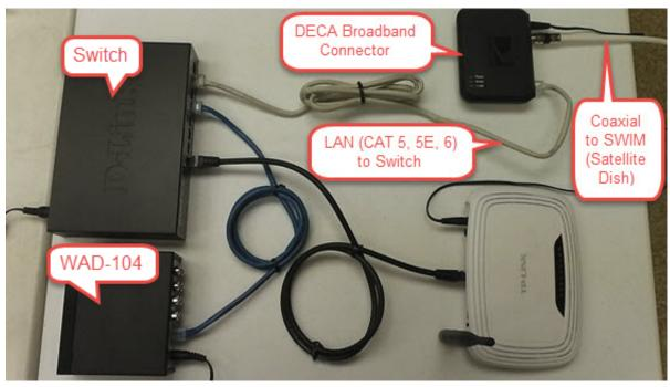
Note that the LAN cable coming from the DECA Broadband Connector to the Switch can be re-routed to connect from the DECA Broadband Connector to any one of the LAN ports in the TPL 740N.
