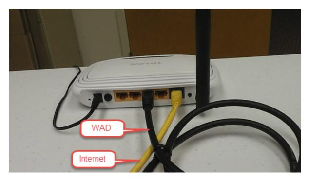
For Auto Channel Naming, connect DECA Broadband Connector as follows. Here we demonstrate using the WAD-104 and a Switch.
